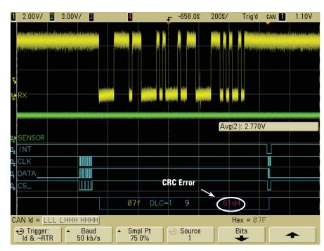
Figure 4: Random errors observed in CAN decode while triggering on data frame ID:  $\rm 07F_{HFX}$
