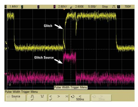
Figure 7: Pulse-width triggering reveals source of random and infrequent glitch
