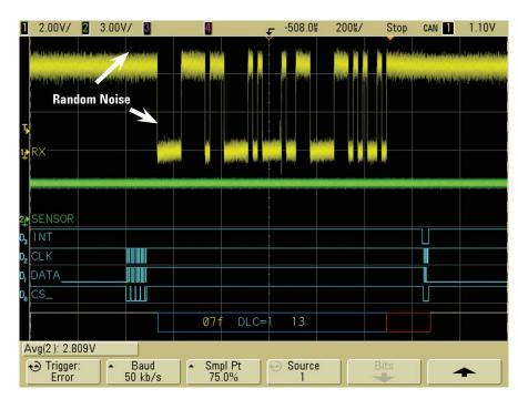
Figure 5: Triggering on CAN error frames isolates acquisitions on bad frame transmissions
