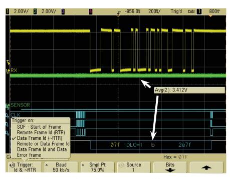
Figure 3: Capturing multiple SPI and CAN signals using an MSO with CAN triggering and decode
